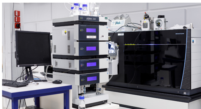
Orbitrap Eclipse coupled online to an Ultimate 3000 nano-HPLC
